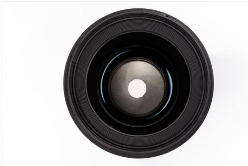
Aperture is like the “pupil” for your camera system, which can open and close to change the amount of light that passes through. Note the nine blades in this lens, which form a diaphragm to block any light that tries to pass, except through the center.
